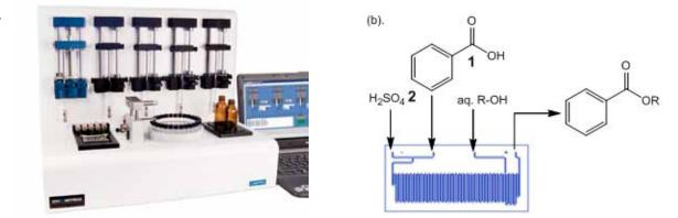
Figure 1. Illustration of (a). Labtrix<sup>®</sup> S1 the micro reactor development equipment used in this investigation and (b). a schematic of micro reactor (3023) set-up employed.
