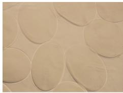
Figure 2: Light microscope image at  $10 \times$  displaying egg shaped pectin-oligochitosan microbeads. Hardening bath strongly stirred.
