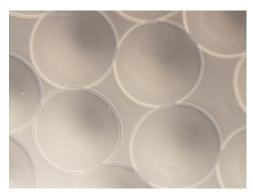
Figure 1: Light microscope image at  $10 \times$  displaying spherical pectin-oligochitosan microbeads with a size of  $500 \pm 20 \mu m$ . Hardening bath gently stirred.
