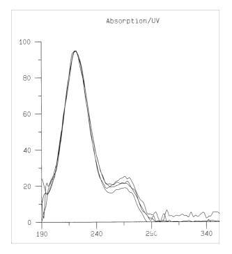
Fig. 12: In situ UV-spectra of 20, 50 and 100 ng Atrazine plotted together with the spectrum of the component in the sample, corresponding to 0.08 µg Atrazine per liter. All spectra are in an acceptable accordance.
