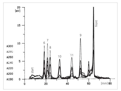
Fig. 7: Calibration mixture 2, gradient A, 50 ng each component; 6 = Metoxuron, 7 = Monuron, 8 = Chlortoluron, 9 = Propazine, 10 = Phenmedipham, 11 = Metobromuron
