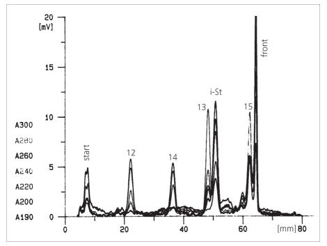
Fig. 9: Calibration mixture 3, gradient B, 50 ng each component; 12 = 2,4-D, 13 = Atrazine, 14 = Metazachlor, i-St = Benzanilid, 15 = Pendimethalin
