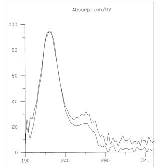
Fig. 13: In situ UV-spectrum of component 3 in fig. 8, corresponding to 0.05 µg Simazin per liter, plotted together with the spectrum of 20 ng Simazin (calibration substance). The accordance is satisfying.
