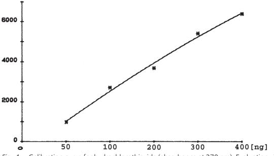
*Fig. 4* Calibration curve for hydrochlorothiazide (absorbance at 270 nm): Evaluation via peak height with 2. degree polynomial. Calibration range 100-800 ng, corresponding to 0.2-1.6 mg/L.
