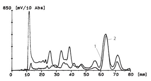
*Fig. 3* Densitogram at 270 nm (1) and at 540 nm after derivatization (2). Hydrochlorothiazide, which was identified by UV- spectra, has reacted to an azo dye by derivatization.
