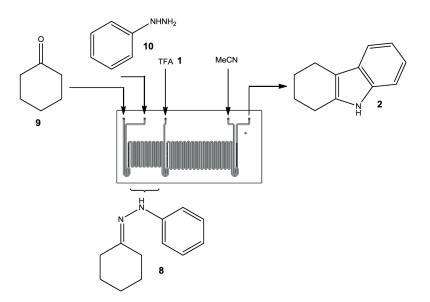
**Figure 5.** Schematic illustrating the device (3224) employed for continuous flow indolisation of an *in-situ* synthesised hydrazone **8**.
