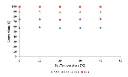
**Figure 3.** Graph illustrating the effect of reaction time and temperature on the conversion of 2-ethyl-1hexanol **2** to 2-ethyl hexyl nitrate **1** in Labtrix<sup>®</sup>-S1 Ultra Flex.
