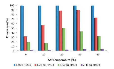
**Figure 2.** Graph illustrating the effect of  $HNO_3$  **3** equivalents (eq.) on the formation of an aliphatic nitro ester **1**.
