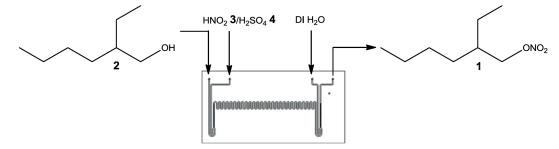
**Figure 2.** Reactor manifold (3222; Volume 5 μl) used to assess the continuous flow nitration of 2-ethyl-1hexanol **2**.
