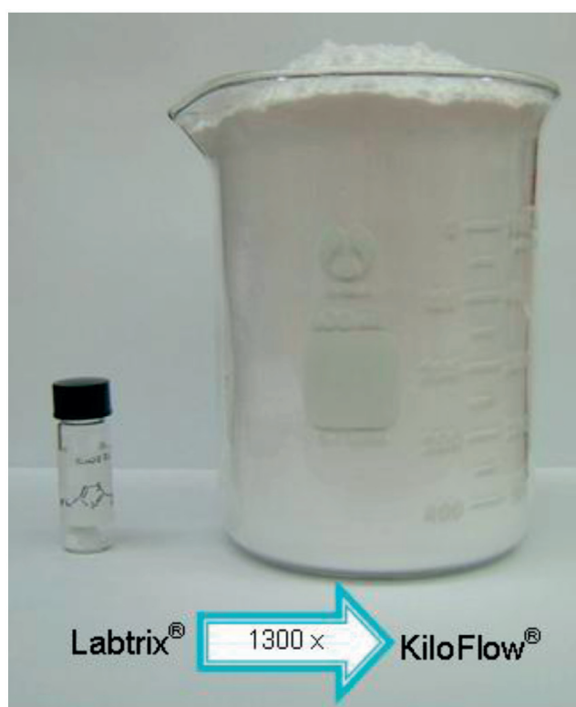
Figure 4. Photograph illustrating the aminothiazole product 1 synthesised in Labtrix® (~100 mg) and KiloFlow® Basic (~1 kg).
