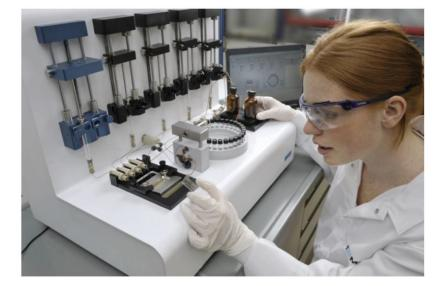
**Figure 1.** Illustration of Labtrix<sup>®</sup>-S1, the automated micro reaction development apparatus developed by Chemtrix.
