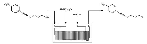
**Figure 2.** Schematic illustrating the Labtrix<sup>®</sup> reaction manifold used for the assessment of nucleophilic fluorination under flow conditions.
