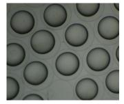
Figure 1: Mono-dispersed, homogenous and spherically shaped liquid-core microcapsules with a DCM-PLA core.
