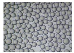
Figure 2: Mono-dispersed and spherical PLA micro-beads of equal shape and size.
