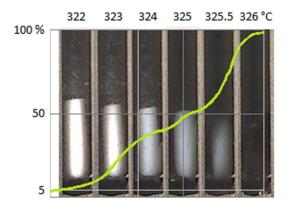
Figure 1. Temperature dependent melting process for PTFE. The green curve illustrates the corresponding melting grade recorded by the Melting Point Monitor 1.2 software. The melting range was observed between 322.9  $\pm$  0.4 °C and 326.0  $\pm$  0.1 °C.
