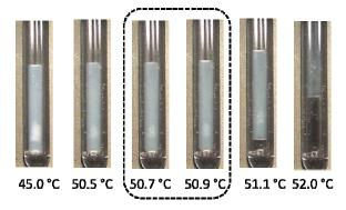
Figure 2. Snapshots of the palm stearin sample during the melting process. The SMP determined for six samples was 50.7±0.1 °C.
