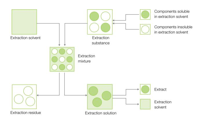
The extraction substance "sausage" is a mixture of meat components in and fat enclosed in these components. The homogenized substance is mixed with a solvent (extraction solvent). This extraction mixture is then separated and insoluble components remain as residue . If this procedure is repeated several times, the proportion of fat in the solvent increases. Pure fat is then obtained by distilling the solvent portion of the mixture.
