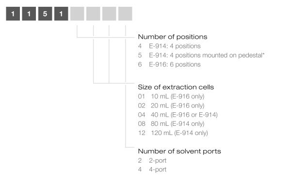
\*Recommended for the use of round bottom flasks and Analyst R-6/Polyvap R-6 collection vessels; SpeedExtractor E-914 (Order number 11515xxx) is mounted on a pedestal which heightens the unit by 50 mm. The pedestal cannot be upgraded on existing instruments
